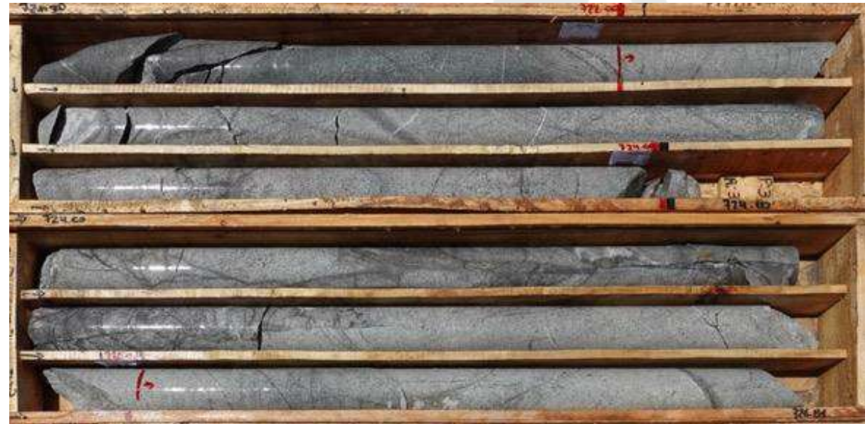
Hole PIU07: Brecciated and veined diorite porphyry with sericite-pyrite and kaolinite alteration associated with high sulfidation vein and breccia mineralization
